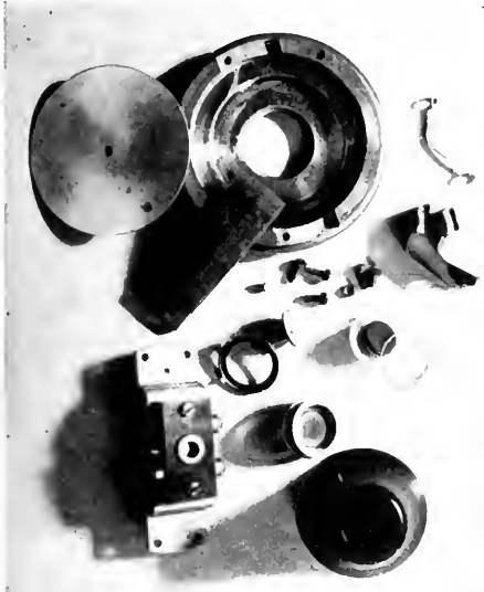
FIG. 28.—WESTERN ELECTRIC SUPPLY CO TRANSMITTER DISSECTED.
